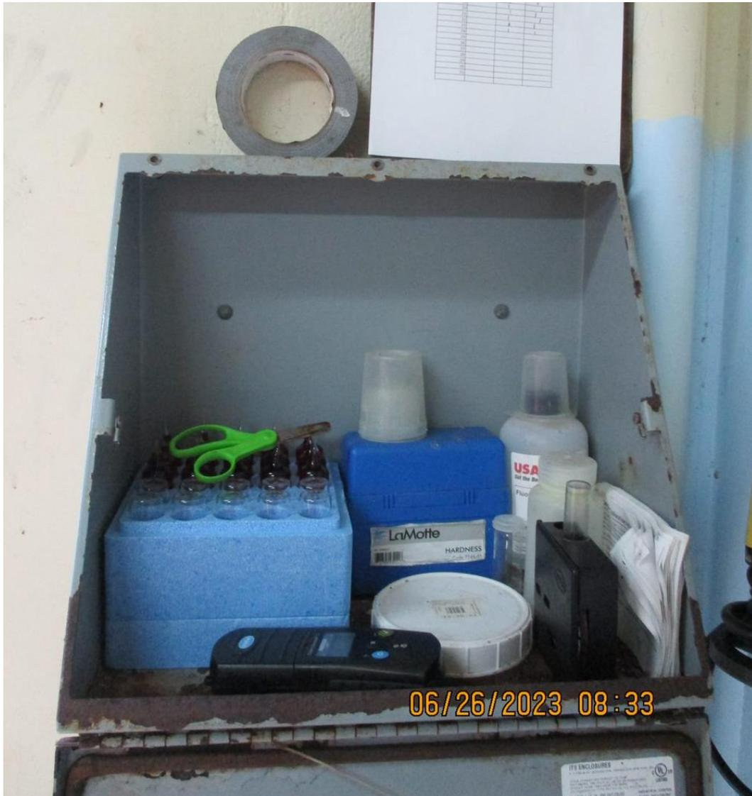
**Figure 11.** Chemical testing equipment and reagents
