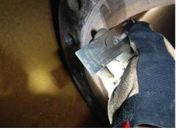
F24) **Finding:** Minor pipe pitting was ide ed on (b) (3) (A) lateral pipe below a bubbled coating (between pipe support (b) (3) (A) Piping is (b) (3) (A) Pitting depth of 0.030" to 0.070" was noted.
