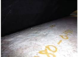
B30) Pitting Corrosion on (JP-5 line) between (158" from at 6 o'clock. Corrosion Area is 10" x 10", Pit Depth is 0.055" - 0.102", Metal thickness on unaffected area is 0.218" - 0.238" resulting in a remaining metal thickness of 0.116" to 0.136". Note: very close to API 574 (0.110") and ASME 31.3 (0.109" limits).
