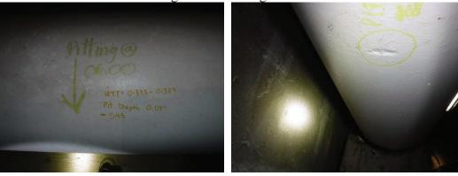
B35) Inactive pitting on F-76) line between (22" from ) at 6 o'clock. Corrosion Area is 15" x 24", Pit Depth is 0.050" - 0.114", Metal thickness on unaffected area is 0.386" - 0.393" resulting in a remaining metal thickness of 0.186" to 0.193".
