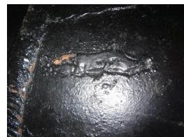
B12) **Finding:** Nonstandard flange configure on (blind flange) noted on the (b) (3) (JP-5) line near (b) (3) . A 12- welding neck-flange with flat plate welded is used. Note: ASME B16.5 NPS 12 class 150 blind flange has a minimum flange thickness of 1.190". The center plate in the current configuration has thickness of 0.933".
