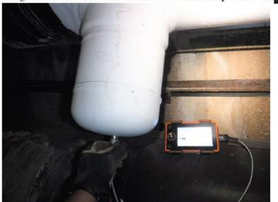
Thickness testing was conducted at all branch welds when it is located near the bottom of the pipe at all locations to inspect for microbial induced corrosion (MIC)
