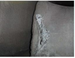
B44) Out-of-round/flat spot noted on the weld (12 o'clock to 3 o'clock position).
