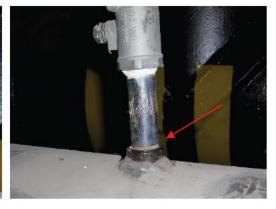
F14) **Finding:** There are eleven mechanic dents identified in this segment of piping inspected. Dents range from minor to moderate (0.030" to 0.950" depth). There is one dent (A-MD-2) identified at that a depth of 0.950" with coincident features (corrosion with multiple gouges). Dents identified are listed in Table F.
