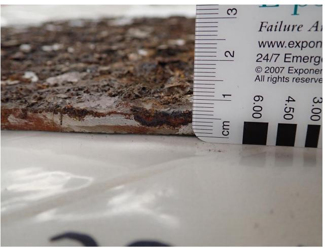
Figure 1: Edge of Coupon #7. Image from non-Navy source alleging the thickness of the remaining steel at the location shown alleging thickness less than the Navy's predictions.
