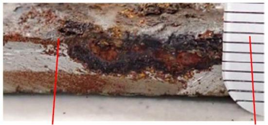
Figure 2: Image taken after coupon removal, prior to receipt by lab. What appears to be a deep corrosion pit was actually rust-covered staining of the edge surface.
