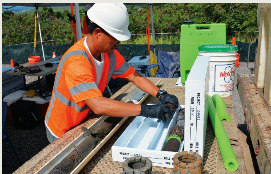
During the rock coring phase, core samples are carefully removed from the borehole and quickly handed off to geologists at 5-foot intervals. Geologists then observe and catalog the cores in order to develop a better understanding of the subsurface geology of the borehole.
