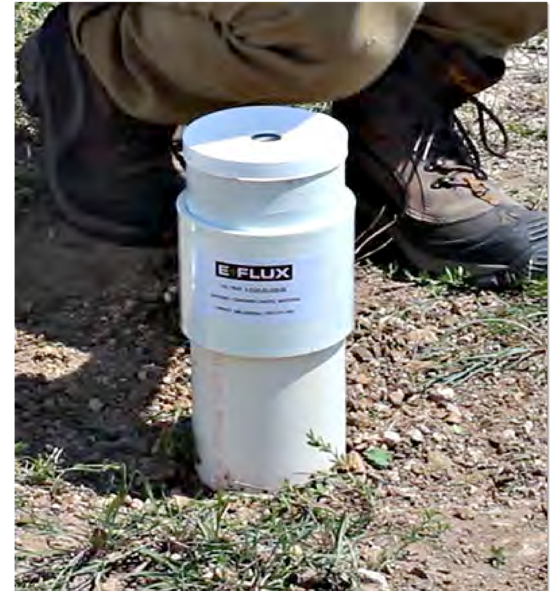
Photo of an installed E-Flux carbon trap sampler. http://soilgasflux.com
